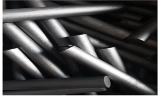
SAE – 4320H. No scale seen after shot blasting
