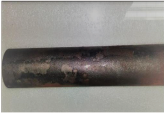
SAE – 4320H. Adherent scale seen after shot blasting
